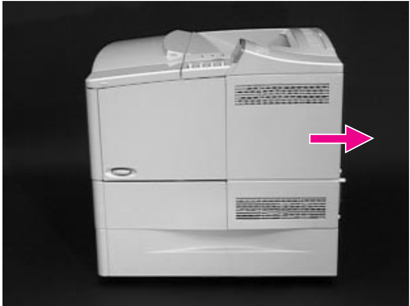
Figure 6-2 Removing the Rear Right Side Cover
